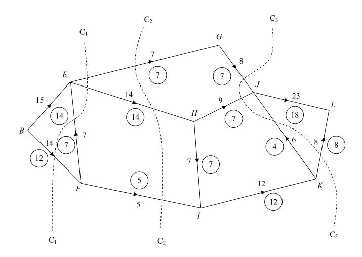
Figure 1 shows a network of roads represented by arcs. The capacity of the road represented by that arc is shown on each arc. The numbers in circles represent a possible flow of 26 from B to L.
