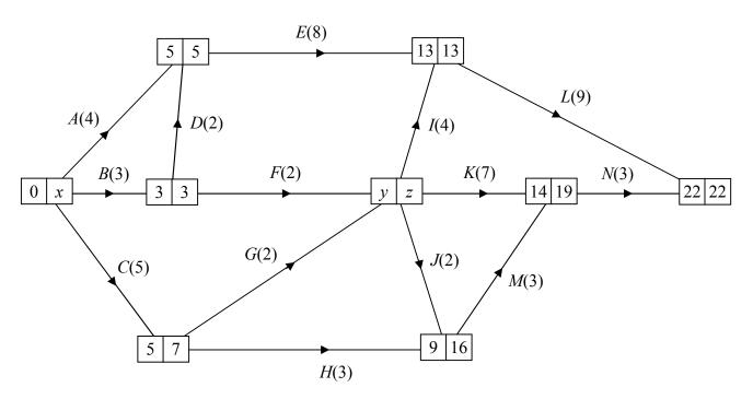
A trainee at a building company is using critical path analysis to help plan a project. Figure 4 shows the trainee's activity network. Each activity is represented by an arc and the number in brackets on each arc is the duration of the activity, in hours.
