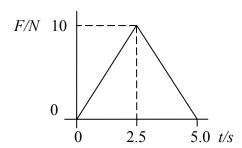
A force, *F*, varies with time, *t*, as shown by the graph and is applied to a body initially at rest on a smooth surface. What is the momentum of the body after 5.0 s?
