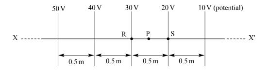
The diagram shows how the electric potential varies along a line XX' in an electric field. What will be the electric field strength at a point P on XX' which is mid-way between R and S?
