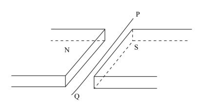
A wire lies perpendicularly across a horizontal uniform magnetic field of flux density  $20 \times 10^{-3}$  T so that 0.30 m of the wire is effectively subjected to the field. If the force exerted on this length of wire due to a current in it is  $30 \times 10^{-3}$  N downward, what is the current in the wire?
