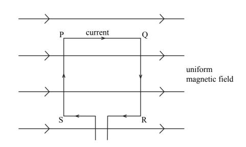
The diagram shows a square coil PQRS placed in a uniform magnetic field with the plane of the coil parallel to the lines of magnetic field. A constant current is passed round the coil in the direction shown, causing a force to act on side PS of the coil. Which one of the following statements about the forces acting on the other sides of the coil is correct?
