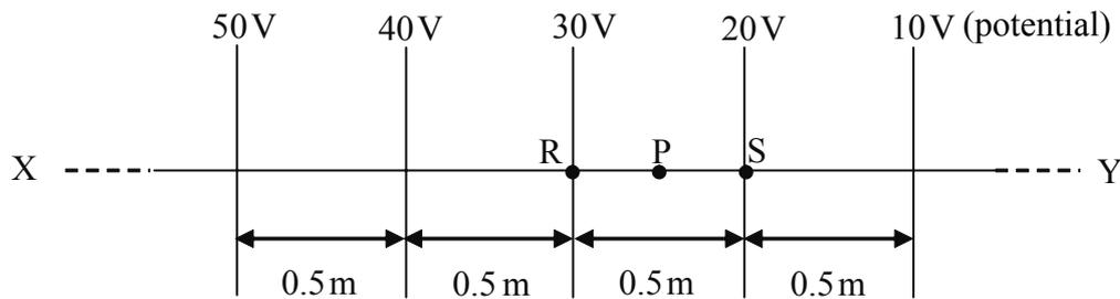
The diagram shows how the electric potential varies along a line XY in an electric field. What will be the electric field strength at a point P on XY, which is mid-way between R and S?
