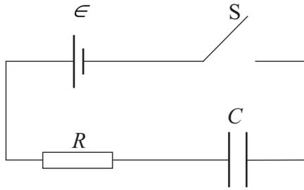
When switch  $S$  is closed, the capacitor of capacitance  $C$  begins to charge from the cell of emf  $\epsilon$  through the resistor of resistance  $R$ . The initial current in the circuit is  $I$ .
